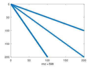
Figure 22.3: Structure of simple sparse matrix.
