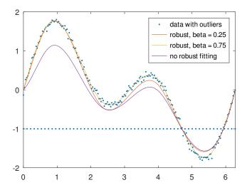
Figure 28.5: Comparison of two different levels of robust fitting (beta = 0.25 and 0.75) to noisy data combined with outlying data. A conventional fit, without robust fitting (beta = 0) is also included.
